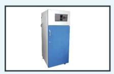
Double walled construction outer body made of MS, duly powder coated and inner SS/Alu. With front door having a glass window to inspect the samples placed inside the chamber. Temp. range from ambient  $+5^{\circ}$ C to  $60^{\circ}$ C with an accuracy of  $\pm 1^{\circ}$ C. Temp. humidity controlled by digital temp. controller cum indicator LED(dual display) from 40% to 90% with sensitivity of  $\pm 3\%$  without hygrometer power supply 220/230V.
