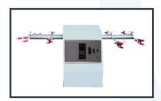
Heavy MS body duly powder coated having two side arms with suitable flask holding clamps, using AC/DC gear motor and shaking speed range 50-250RPM with variable speed control.
