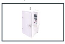
Temperature from  $5^{\circ}$ C.above ambient to  $60^{\circ}$ C Thermostatic control with a sensitivity of  $\pm 1^{\circ}$  C. Double walled- outside made of mild steel beautifully powder coated inside aluminum/Stainless steel, having additional glass door inside. Complete with shelves. To work on 220/230v A.C. Supplied with or without air circulating fan but without thermometer.
