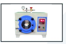
Vacuum oven commonly using the temp. from 50o to 250o. The inner chamber is made out of SS and outer MS with powder coating. Glass wool insulation will be provided all around the inner chamber to minimize the heat loss. The SS door is fitted with a glass window to view the samples placed inside. The temp. is controlled and indicated by a digital temperature indicating controller. Vacuum control valve with a vacuum gauge is also provided. Max. vacuum: 760mm of Hg.
