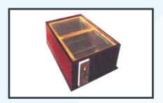
Outer made of wood with PU coating and inner made of copper sheet, epoxy coated and filled with ceramic wool. Inner chamber can accommodate 100 tube of media at a time. Arrangements for water in, out and overflow are equipped with the unit. Temperature is controlled by thermostat, temp. range ambient +5°C to 60°C
