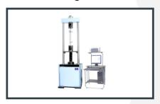
Body made of heavy gauge mild steel with powder coated. It is commonly used for the test of the Gule shear strength, Modulus of Rupture (MOR) and Modulus of Elasticity (MOE) samples in plywood and textile industry.
