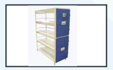
This Tissue culture rack is made of MS/Aluminum pipes powder coated, rack size 120cm X 53cm. Height between each rack is38cm. Each rack is fitted with 2 no. fluorescent tubes and one UV germicidal tube and caster wheel at its base. Each tube has separate ON/OFF switch. 0 – 24 hrs. weekly cyclic timer also equipped with the unit for controlling all the tubes inside the racks.
