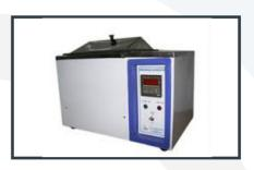
Temperature range from ambient temperature to  $100^\circ$ . Thermostatic control with an accuracy of  $\pm$  1° C. Double walled construction outside MS sheet duly powder coated, inside Stainless Steel . The gap between the walls insulated with glass wool. Bath consist of two pilot lamp, temperature control knob, and ON/OFF switch to work on 220/230volts A.C. Supplied without stirring arrangement rack and thermometer.
