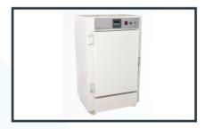
Double walled construction, outer body made of MS sheet duly powder coated, inner made of UV stabilized polycarbonate sheet. Inside the chamber 4 no UV lamp fitted on 4 sides and one no. fluorescent for illumination. When th door closes UV lamp will automatically switch ON and fluorescent lamp will switch OFF and vice versa.
