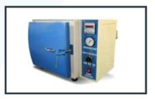
It is a table top front loading autoclave, double walled unit, outer MS powder coated inner 304 grade Stainless Steel. All joints are argon welded. Door is made up of heavy gauge S S sheet and using high quality silicon gasket, used with ISI marked immersion heater 1.5 KW in 230/240V.
