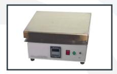
The working space is made of mild steel plate, heating is accomplished by Nichrome heaters provided immediately beneath the working surface. One no. 3 heat control switch will be provided to work the heater either at low or high supplied complete with plug and cord for operation on 230 Colts 50 c/s single phase Mains.
