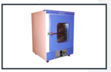
Temperature from  $5^{\circ}$ C.above ambient to  $60^{\circ}$ C Thermostatic control with a sensitivity of  $\pm 1^{\circ}$  C. Heating elements are placed in the ribs at the bottom and sides. Double walled- outside made of mild steel beautifully powder coated with perforated adjustable shelves – thermostat, two indicators and on/off switch. To work on 220/230v A.C. Inside chamber of Anodized aluminum/Stainless steel,
