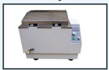
Double walled construction: outer body MS duly powder coated and inner made of SS 304 grade sheet. Temp. is controlled by microprocessor based digital temperature controller, temp. range of  $+37^{\circ}\text{C}$  to  $56^{\circ}\text{C} \pm .5^{\circ}\text{C}$  with audio visual alarm for low and high temperature. Removable SS tray with partition for holding 12 bags. The unit is to work in 220/230 V AC.
