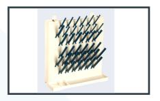
It is used for drying laboratory glassware quickly and safely. By providing continuous warm air circulation through 12/24 hollow drying pegs with large or small bores with dust free filters labware is never too hot to handle. A time proportional high/ low heat controlled with an automatic thermostatic safety control cut off system.
