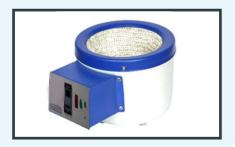
Mantle is made from fiber yarn and good quality nichrome/kanthal wire element. Mounted in a powder coated MS body with glass wool insulation. Fitted with energy regulator. Temp range 100°C.
