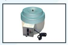
Double walled construction inner made of SS and outer made of MS duly powder coated. The gap between the walls filled with glass wool insulation and the temperature is controlled by thermostat from ambient +5°c to 80°C having an accuracy of +1°C and without thermometer.
