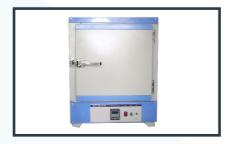
Temperature from +50°C. to 250°C Thermostatic control with a sensitivity of 1°C. Heating elements are placed in the ribs at the bottom and sides. Double walled-outside made of mild steel duly powder coatedwith perforated adjustable shelves, thermostat, two indicators and on/off switch work on 220/230v A.C. inside chamber of anodized Aluminum/Stainless steel - Supplied with or without air circulating fan but without thermometer.
