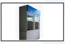
Thick wooden board fabricated, outer surface is finished with laminated mica and inner surface is FRP coated, designed so as to throw all toxic /harmful vapors, thus protecting costly instruments and the persons working the lab. The working table is covered with acid/alkali resistant tiles/FRP or granite slab 20mm thick provided with swan type water tap and v
