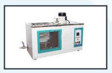
It is used to maintain the correct temperature for estimating kinematics viscosity of oil and petroleum products.
