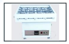
This shaking machine can accommodate khan racks, bottles or flasks of different sizes, DC motor with variable speed and speed regulator 50 to 250 RPM.
