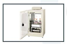
Orbital shaking incubators are specially designed to have combined advantage of a closely controlled incubation/ storage temperature with orbital shaking necessary for many laboratory procedures such as tissue cultures, fermentation studies, enzyme reactions, controlled purification and ageing studies etc.
