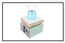
The body fabricated with MS sheet duly powder coated having SS top housing series of magnetic stirrers are most compact models. These are smooth running apparatus utilizing the rotating magnetic field from a balanced permanent magnet (stirring speed – 1200RPM approx..) to induce various stirring action in close or open non magnetic containers. Stirring is
