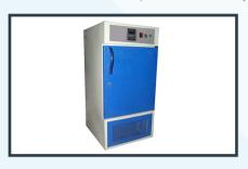
Temperature Ranges from  $5^{\circ}$ C. to  $60^{\circ}$ C with an accuracy of  $\pm.5^{\circ}$  C. Double walled- inside Anodized aluminum/Stainless steel, and outside of mild steel beautifully powder coated with electronic digital temperature controller cum indicator and air circulating fan – transparent door inside – self supported and adjustable perforated racks-magnetic
