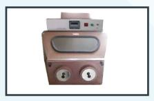
Made of wood with glass panels on the two sidesand back and bottom of the hood are made of good quality plywood properly painted the hood is provided with a hinges transparent front door – the will have a front bottom panel , made of transparent acrylic having two glove compartment s-complete with UV lamp, I no. fluorescent light (20 watts) both
