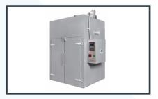
Industrial oven is, triple walled construction outer made of MS sheet, properly painted, second & third wall is made of GI sheet and insulated mineral wool, temperature range from 50°C to 250°C with an accuracy of ±3° C controlled by micro process based digital temperature controller. Provided with an air circulation fan. Supply 415V AC 50 HZ.
