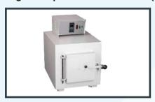
High temperature muffle furnace with maximum temp. 1200°C and working temperature 1100°C. It is controlled by microprocessor based digital temp. Controller fitted with thermal fuse and thermo couple with ceramic wool insulation.
