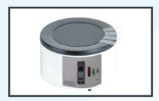
Double walled construction inside made of aluminum, outer made of MS sheet duly powder coated. Temperature is controlled from ambient +5°C to 80°C by Thermostat and without thermometer.
