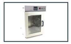
Double walled construction, outer body made of MS duly powder coated, inner chamber made of SS sheet, 304 grade, glass wool insulation, temp. range ambient +5°C to 60°C. Temp. is controlled with microprocessor based digital temp. controller cum indicator. Provided SS tray with suitable support to hold rack or flasks on it. The up and down oscillation can be controlled by an electronic speed regulator, max. 90 stroke/ minute. An air
