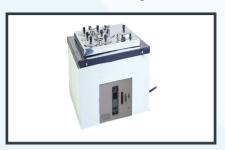
Double walled construction, inner chamber made of SS 304 quality sheet. Thermostatic temperature control, from ambient  $+5^{\circ}$ C to  $80^{\circ}$ C with an accuracy of  $\pm 1^{\circ}$ C. The bath is insulated by 25mm glass wool. 6 holes are provided to accommodate SS pots having 63mm dia X 65mm depth. 2 holes of 30mm dia. to insert tubes.
