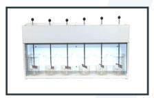
Continuous duty DC motor connected with gear chain arrangement to achieve uniform speed in all spindles SS stirring shaft with adjustable height, illuminated fluorescent diffused light. Supplied with out glass beaker. Stirrer can be controllable from 30 to 250 RPM.
