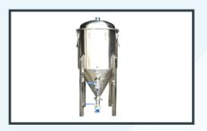
Fermenter is made of triple wall, inner tank made of 3mm thick stainless steel plate, insulated with 20 SWG SS sheet lid and flange will be made of 6mm SS plate and bolted with neoprene gasket.
